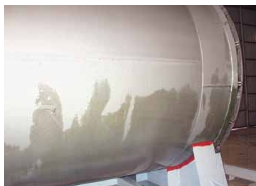
Avesta FinishOne™ Passivator 630- removes free iron (the brown staining seen on the photo).
